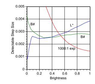
Figure 10: Detectable step size of the B# scale compared to two others over their brightness range.
