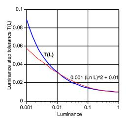
Figure A1-1: Luminance step threshold data and approximating function.
