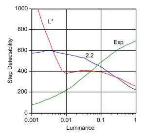
Figure 8: Step "detectability" d(L)/T(L) of three gray scales.
