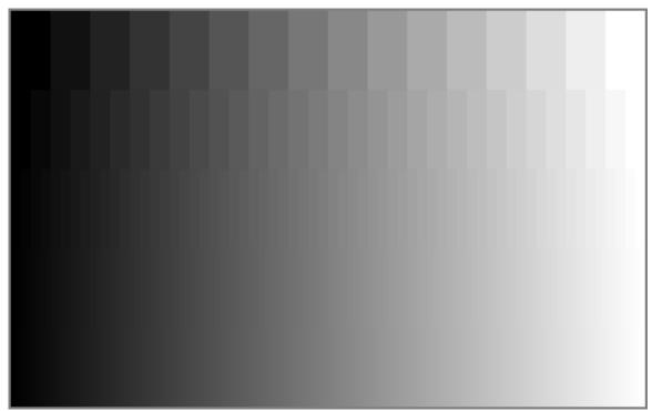
Figure 6: Progressively increasing samples of the gamma 2.2 scale
