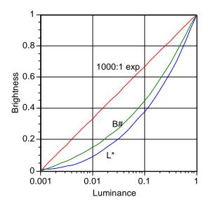
Figure 9: Brightness index of B# compared to two other scales as a function of luminance.
