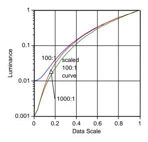
Figure 19: The effect of simple scaling of a low contrast response to a higher one.
