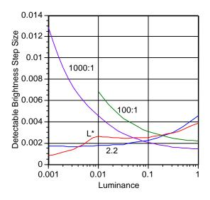
Figure 7: Just noticeable brightness step for four scales as a function of luminance
