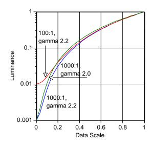
Figure 20: Scaling gamma between different contrast media.
