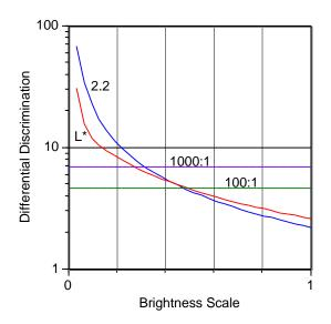
Figure 2: Differential discrimination function of the candidate uniform brightness scales, plotted against brightness.
