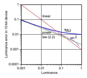
Figure 13: 10-bit device luminance errors compared to the human visual step tolerance, T(L).
