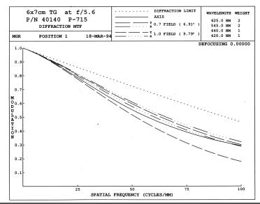
Modulation transfer function. The exact glass type, surface design, and alignment of the lens elements, all contribute to the overall sharpness of the resulting image. The MTF performance curve embodies how well a lens can reconstruct spatial frequencies at its image plane. A figure of merit for a lens is the frequency which can be imaged at a 50% contrast level, the spatial bandwidth of the lens.
