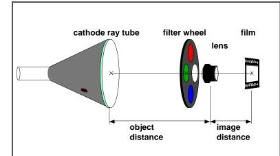
Typical CRT film recorder optical path. The four elements illustrated here are present in some form in all film recording equipment. A diverse range of technology has been applied to the problem of recording images on film; CRTs are a dominant choice due to their relatively low cost. The demands on the writing equipment are high because the media, silver-based film, is so capable and its performance continues to improve.
