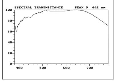
Lens transmission and scattering. Most lens elements are quite clear across the visual spectrum. The antireflection coatings on the other hand, tend to favor certain wavelengths over others, and many glass types start to exhibit scattering at the blue end of the spectrum. The result of these effects is to introduce a slight tint to the flare associated with the lens.
