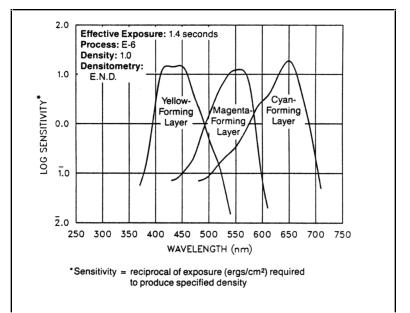
Sensitivity relative to the exposure spectrum. Here are the sensitivity curves superposed on the spectral components of the color separated CRT phosphor. It is desirable to have the exposure energy in each band match the corresponding sensitivity function without influencing the other layers of the film.
