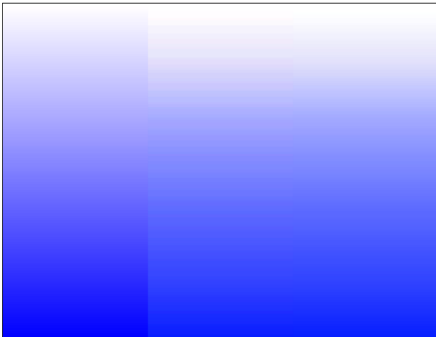
Figure 15. Left: simple RGB to CMY, center: color managed ramp with inadequate profile precision and excessive noise content, right: improved color processing. The color signals have been amplified by 2 for this illustration.
