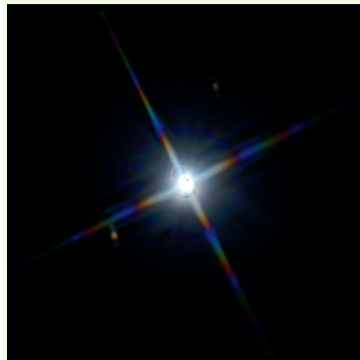
d) A rendering of Vega. The colored diffraction spikes are an artifact of the sensor's color sampling mosaic. The loops and contours at the core are a result of imperfect de-blurring and alignment. The 9th and 10th magnitude stars are visible in the same view as Vega, a 0-magnitude beacon. This scene shows a dynamic range of objects whose brightness differs by 100,000:1.
